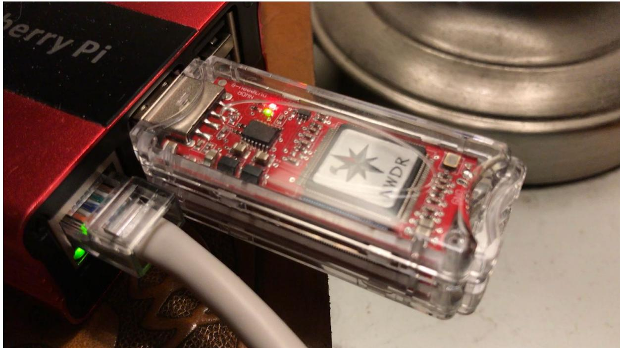
The XLX367 transcoding server: Raspberry 3B+ on wired network with 2 ThumbDV's.
